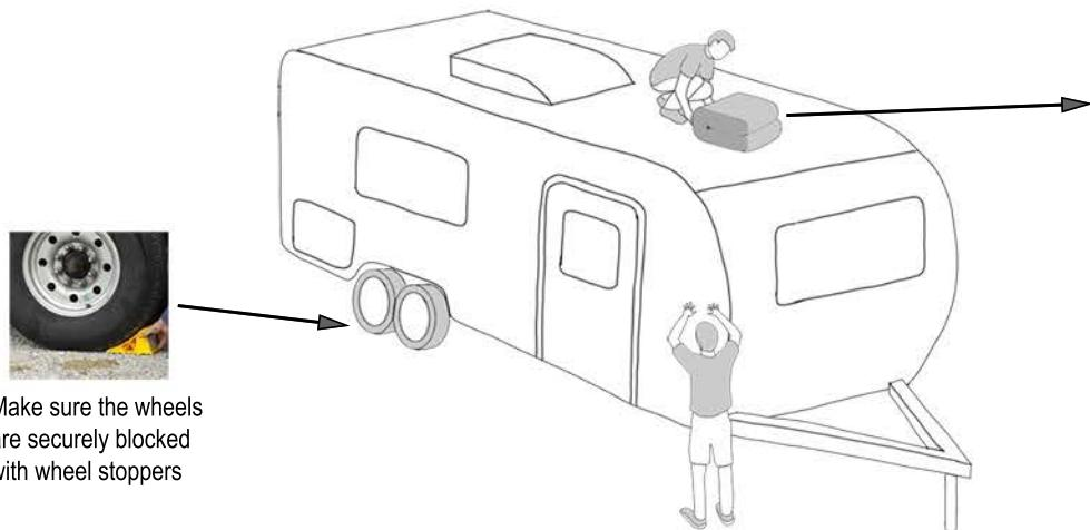
Make sure the wheels are securely blocked with wheel stoppers
